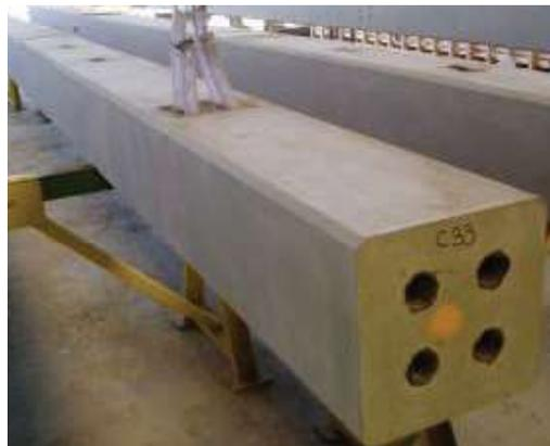
**Figure 20 .** Standardisation of columns is also based on a 50 mm increment, but for the same reasons can be varied.
